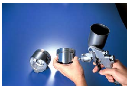
Various methods can be used to apply Molykote Anti-Friction Coatings to entire parts or localized areas. Hand spraying is shown.
